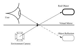
Fig. 3: Environment Mapping for Planar Objects
