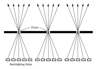
Fig. 5: Integral Display using Backlighting Modulation.
