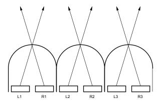
Fig. 4: Stereo Display using Lenticular Screens
