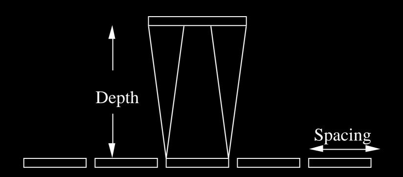
Pixel size = Pixel Spacing + Depth \* Pixel Angle
